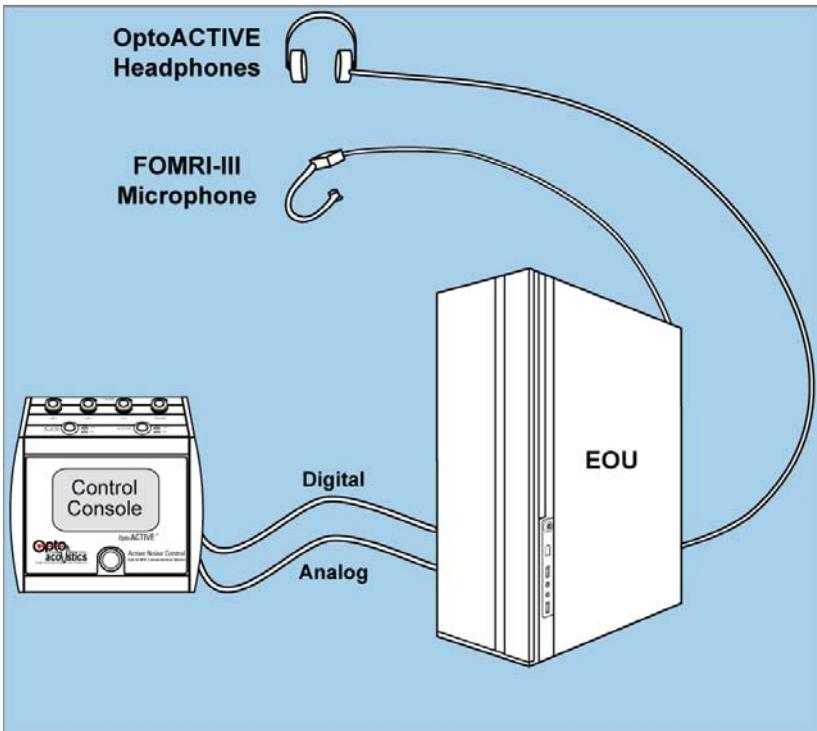
Figure 2-1. *OptoACTIVE Optical MRI Communication System*
