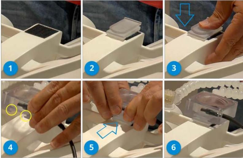
Figure 2-2. *Attaching the FOMRI-III microphone to the coil*
