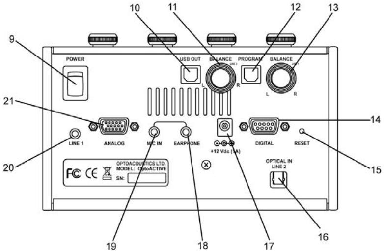
Figure 3-2. Back Panel OptoACTIVE Control Console
